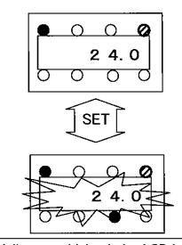
Adjust sensitivity during LCD is flashing, enter with SET switch.
