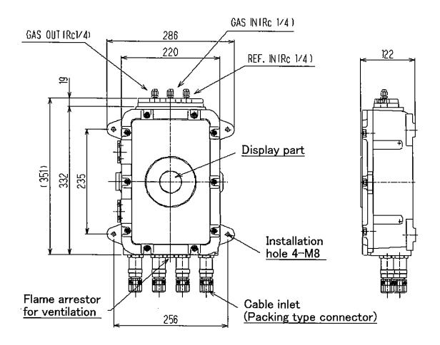
\* Quantity to be used with packing type connector, kind of packing and inner diameter of packing subject to customer's application for use.
