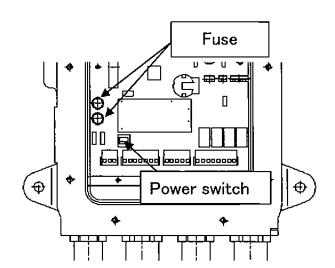
(4) Supply the power source and confirm that the analyzer works in normal.
