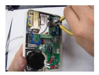
Let cable clamp through the upper part of the hole to pull out cable and fasten the cable clamp halfway.
