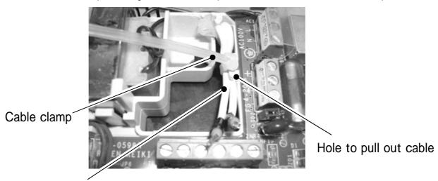
AC cable (Let the cable clamp through beneath of the hole to pull out cable)
