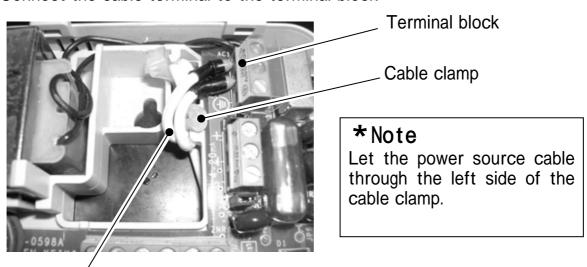
Power source cable (Let the power source cable through the left side of the cable clamp)
