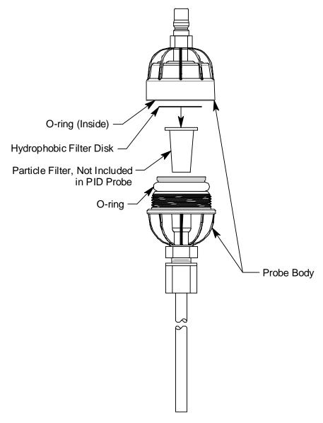
Figure 19: Replacing the Particle Filter and Hydrophobic Filter Disk
