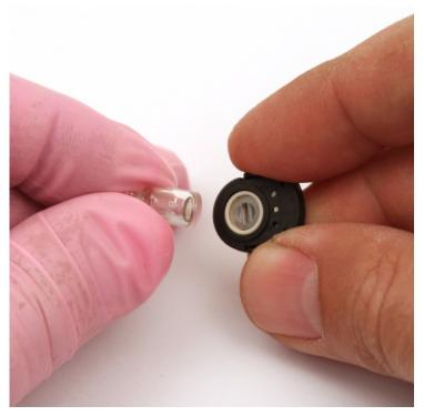
Figure 34: Reinstalling Electrode Lamp
