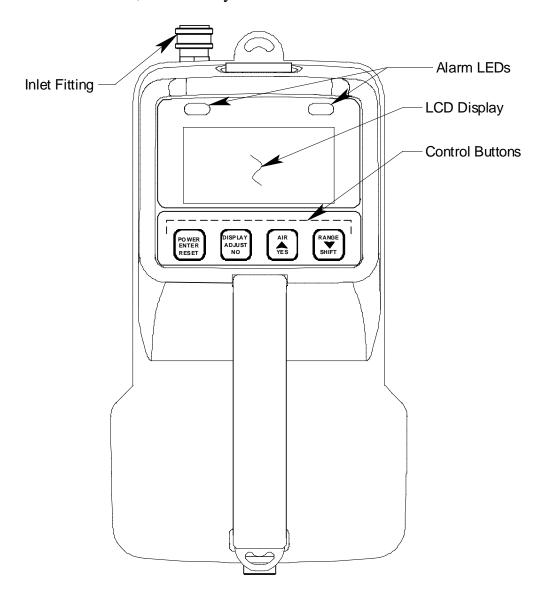
**Figure 1: Component Location, Top View**
