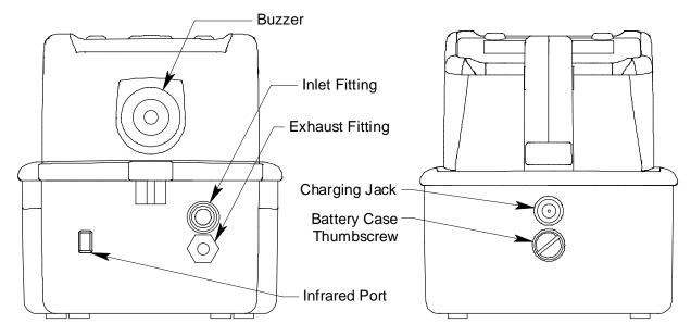
Figure 3: Component Location, Front & Back
