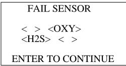
The buzzer and alarm LEDs activate in a double pulsing pattern. Press and release the POWER ENTER RESET button to reset the alarm and continue to the Calibration Value Screen for the infrared hydrocarbon channel. After calibrating the infrared hydrocarbon channel by following the instructions below, attempt to calibrate the standard channels again. If the failure continues, investigate the cause. See "Troubleshooting" on page 70.
