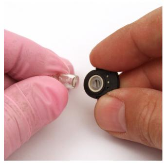
Figure 32: Reinstalling the Electrode Lamp
