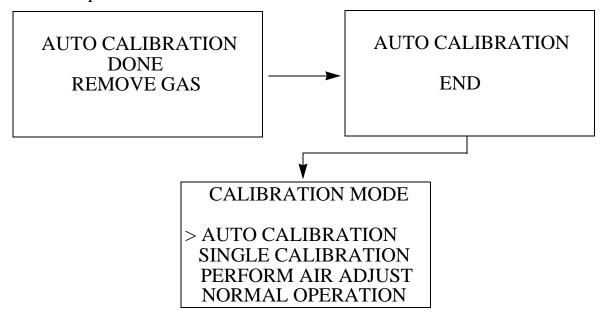
If the infrared  $CO_2$  channel cannot be adjusted to the proper value, a screen displays that indicates a calibration failure and indicates that the infrared  $CO_2$  sensor failed to calibrate.
