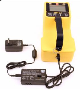
Figure 15: Connecting the EAGLE 2 to the Charger
