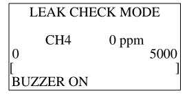
**NOTE:** For maximum sensor stability, allow 3-5 minutes for the sensor to warm up. The small increment size in the lower range of a ppm measurement can cause instability if the unit is not properly warmed up.
