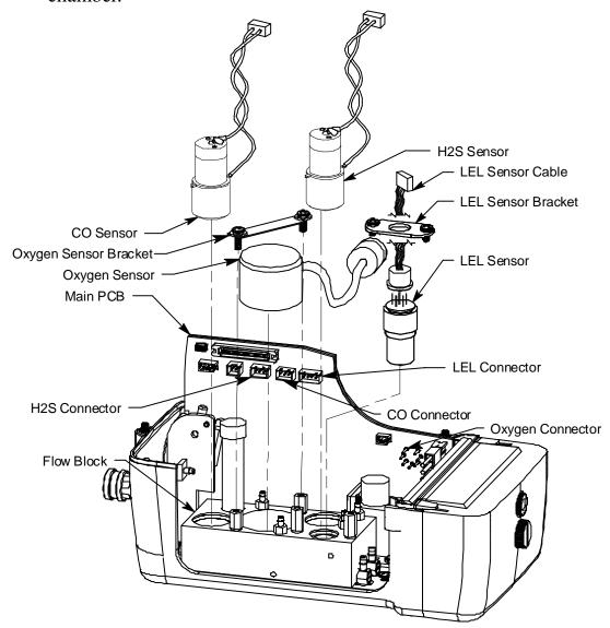
Figure 22: Replacing a Sensor
