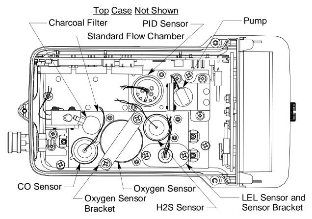
Figure 25: Typical PID Sensor Location
