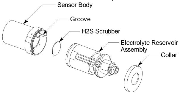
Figure 36: ESM-01 Sensor Component Location
