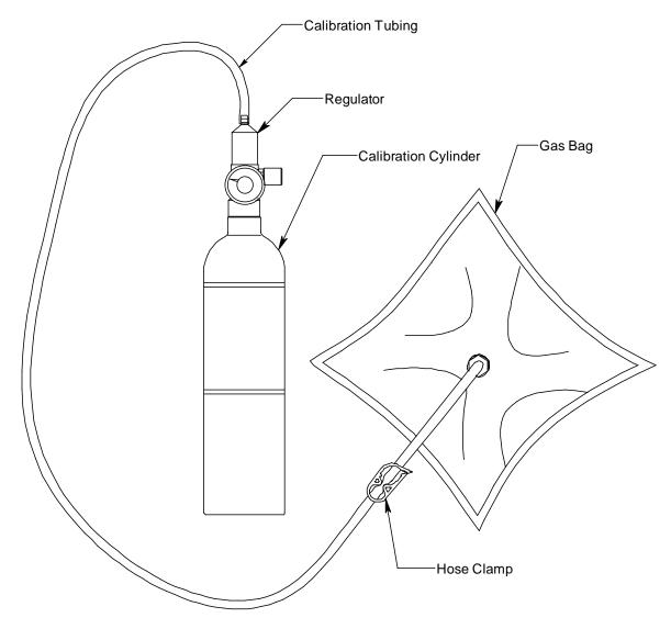
Figure 23: Gas Bag Calibration Kit
