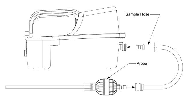
Figure 6: Sample Hose and Hydrophobic Probe
