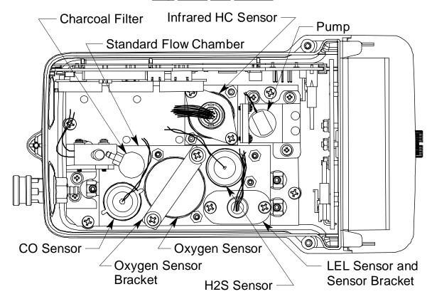
Figure 41: Typical Infrared Hydrocarbon Sensor Location
