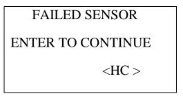
The buzzer and alarm LEDs activate in a double pulsing pattern. Press and release the POWER ENTER RESET button to reset the alarm and continue to the Calibration Mode Screen. Attempt to calibrate the infrared hydrocarbon channel again. If the failure continues, investigate the cause. See "Troubleshooting" on page 70
