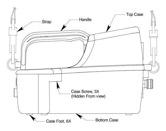
Figure 2: Component Location, Side View
