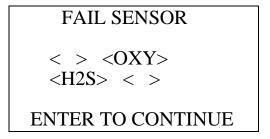
The buzzer and alarm LEDs activate in a double pulsing pattern. Press and release the POWER ENTER RESET button to reset the alarm and continue to the Calibration Value Screen for the infrared CO<sub>2</sub> channel. After calibrating the infrared CO<sub>2</sub> channel by following the instructions below, attempt to calibrate the standard channels again. If the failure continues, investigate the cause. See "Troubleshooting" on page 70
