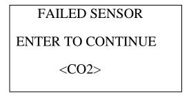
The buzzer and alarm LEDs activate in a double pulsing pattern. Press and release the POWER ENTER RESET button to reset the alarm and continue to the Calibration Mode Screen. Attempt to calibrate the infrared CO<sub>2</sub> channel again. If the failure continues, investigate the cause. See "Troubleshooting" on page 70
