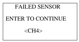
The buzzer and alarm LEDs activate in a double pulsing pattern. Press and release the POWER ENTER RESET button to reset the alarm and continue to the Calibration Mode Screen. Attempt to calibrate the infrared methane channel again. If the failure continues, investigate the cause. See "Troubleshooting" on page 70
