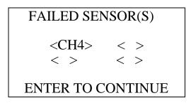
If the catalytic combustible sensor fails, it is not possible to enter Leak Check Mode. Press and release the POWER ENTER RESET button to acknowledge the failure and return to the Mode Select Screen. Replace the failed sensor.
