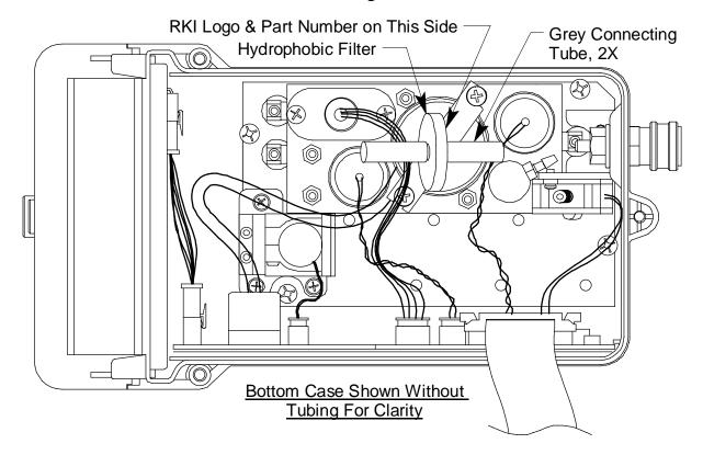
Figure 20: Replacing the Hydrophobic Filter
