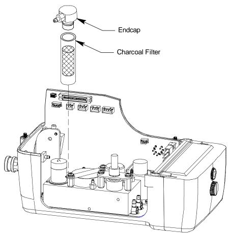
Figure 21: Replacing the Charcoal Filter
