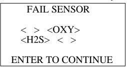
The buzzer and alarm LEDs activate in a double pulsing pattern. Press and release the POWER ENTER RESET button to reset the alarm and continue to the Calibration Value Screen for the infrared methane channel. After calibrating the infrared methane channel by following the instructions below, attempt to calibrate the standard channels again. If the failure continues, investigate the cause. See "Troubleshooting" on page 70.
