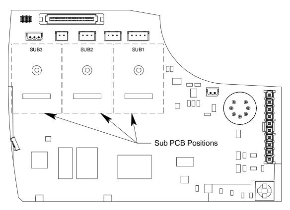
Figure 24: Sub PCB Positions
