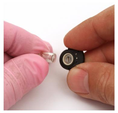
Figure 30: Reinstalling the Electrode Lamp
