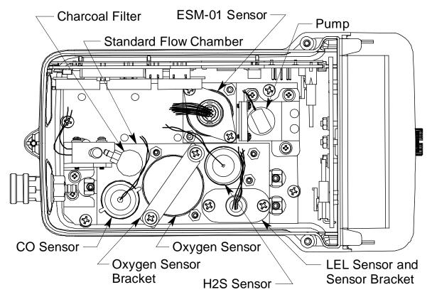
Figure 35: Typical ESM-01 Sensor Location
