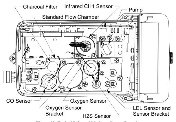
Figure 40: Typical Infrared Methane Sensor Location
