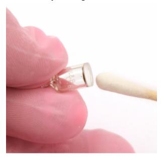
Figure 29: Polishing the Electrode Lamp Window
